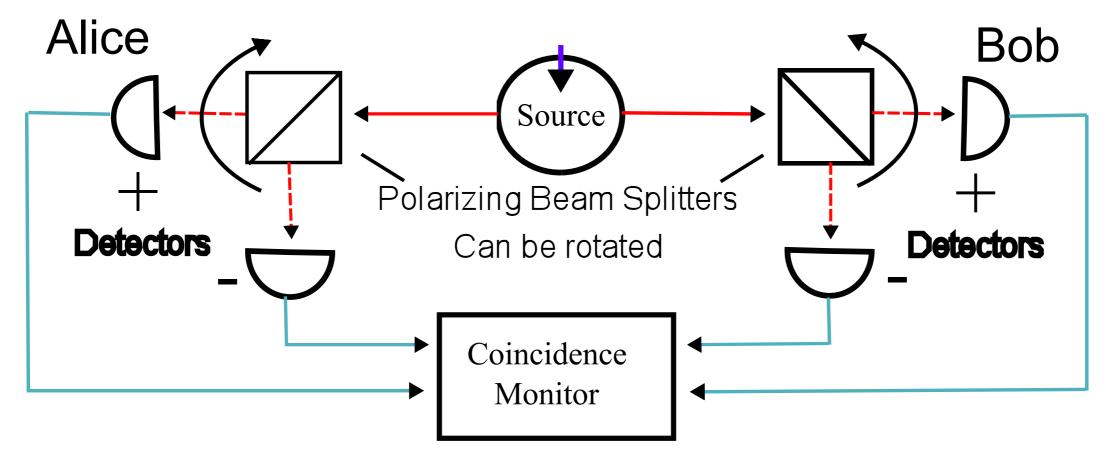
Source can use SPDC (spontaneous parametric down-conversion) for instance to generate pairs of entagled photons
